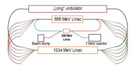
Figure 3: The improved acceleration scheme of FSF.
