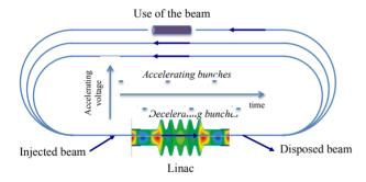
Figure 1: A sketch of a three-pass ERL.
