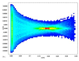
Figure 1: GPT simulated density distribution of 100 keV electron beam with 16pC, conduction angle of  $\pm 20^{0}$
