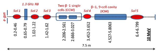
Figure 2. Layout of 10 MeV injector for VECC e-Linac
