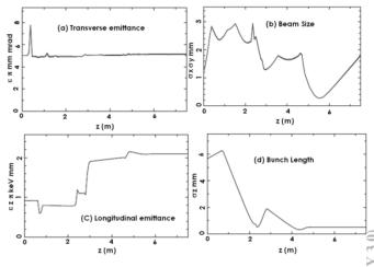
Figure 5. Optimised beam dynamics parameters with  $\pm 16^{0}$  beam;(a) transverse emittance, (b) beam size, (c) longitudinal emittance, (d) bunch length variation along the length.
