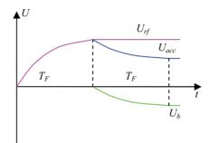
Figure 1: Transient beam loading effect.
