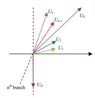
Figure 4: Vector diagram of phase modulated bunch.
