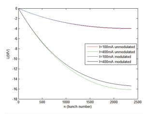
Figure 8: modulated and un-modulated beam loading.
