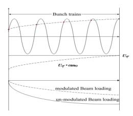
Figure 3: Principle of bunch phase modulation.
