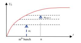
Figure 5: Bunch induced field attenuating with time.
