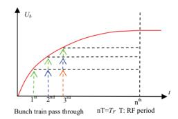
Figure 2: Attenuation and superposition of bunch induced voltage.
