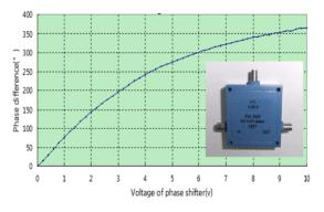
Figure 6: Phase shift vs control voltage
