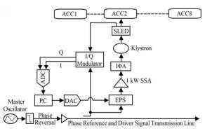
Figure 5: Diagram of phase stability system
