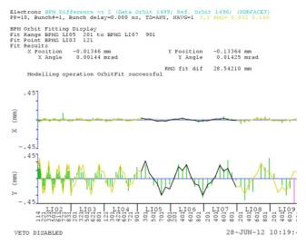
Figure 2: Oscillation data in y, at Li07 501 there seems to be an additional kick pointing to a weaker quadrupole.
