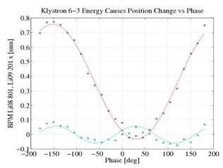
Figure 3: The phase of klystron 6-3 was varied and the resulting downstream orbit observed. At BPM Li09 201 it was up to 800  $\mu m$  and in phase with acceleration, two BPMs earlier, near the zero-crossing, a 100  $\mu m$   $2^{nd}$  harmonic-like effect was seen.
