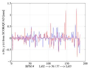
Figure 1: The absolute orbit is steered flat, but the corresponding corrector/quadrupole values for x (blue) and y (red) indicate big bending around 145.
