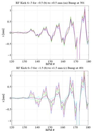
Figure 4: The RF kick of klystron 6-3 (between BPM # 132 and 133) is barely influenced by a bump with the maximum at its front at 301 (top), while at its end at 401 a +1 mm bump cancels the RF kick (bottom). Further downstream seems to be more and more dispersion.
