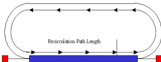
Figure 2: Traditional recirculation geometry.
