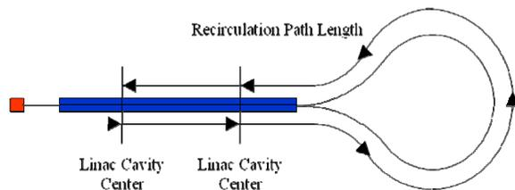
Figure 3: Reflex or herring-bone geometry.
