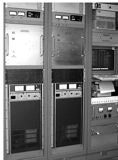
Figure 3. Two amplifiers (center of racks) and monitoring computer on right. DC power supplies are at lower left.
