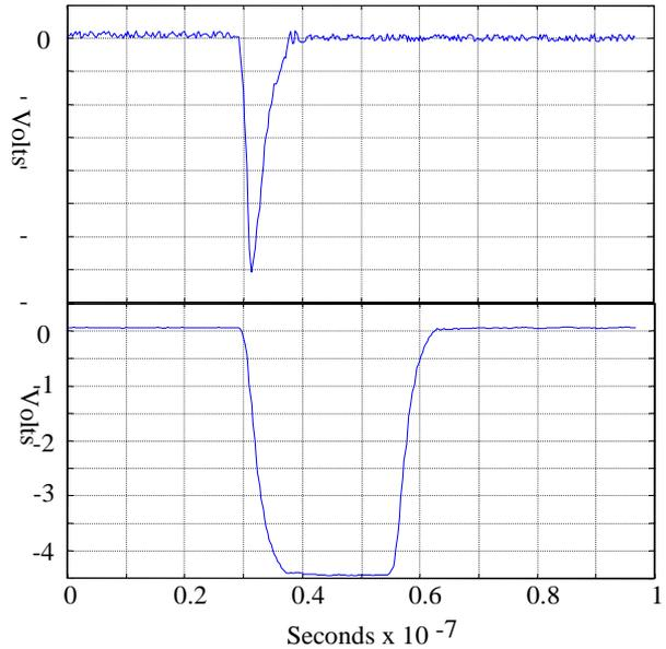
Figure 1: Simulation showing the expected CCLM performance as  $n_b$  is increased from 1 (top half of figure) to 90 (bottom half). The top half of the figure was recorded during SLC operation and illustrates a beam loss of 0.2J.
