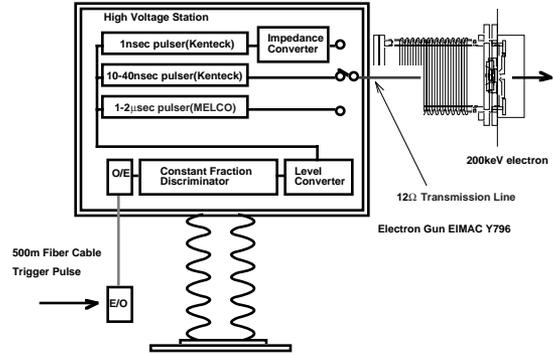
Figure 1: Schematic drawing of the grid pulser system.
