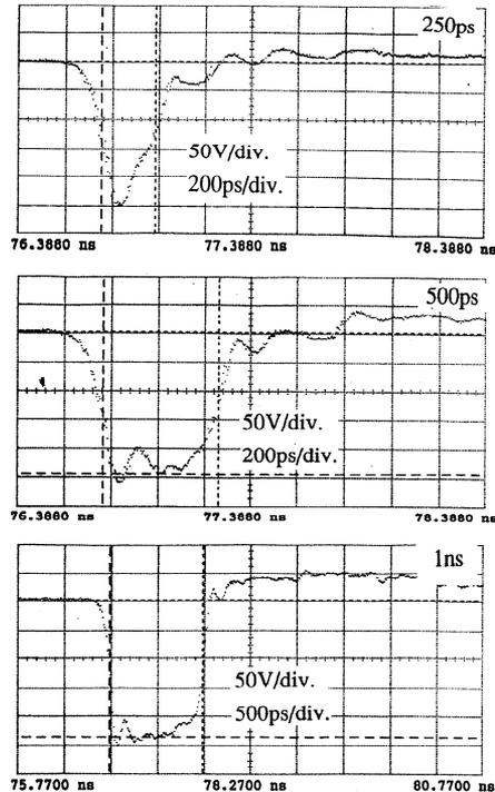
Figure 2: Waveform of three fixed outputs of single-mode grid pulser(250ps,500ps,1ns)
