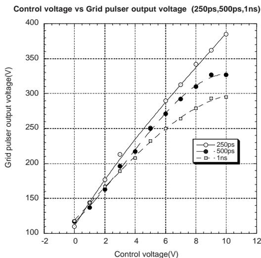
Figure 3: Control voltage vs grid pulser output voltage
