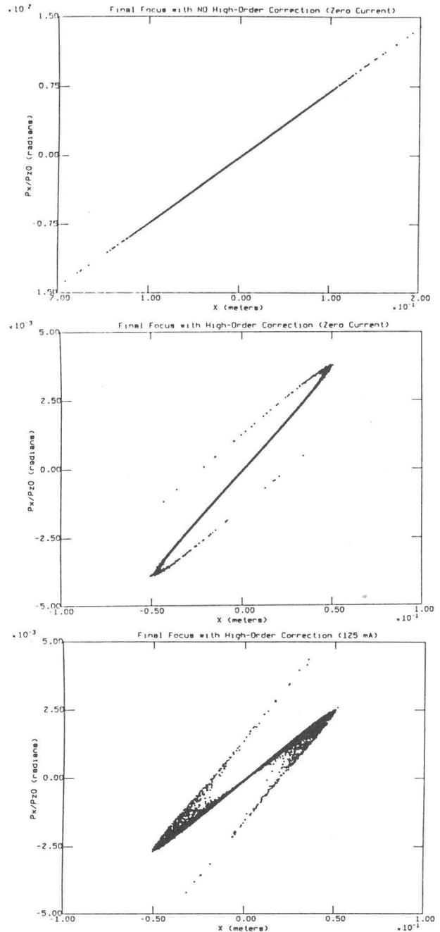
Fig. 3  $X-P_x$  phase space for beam on target without octupoles or space charge (top), with octupoles but not space charge (middle) and with both octupoles and space charge (bottom).
