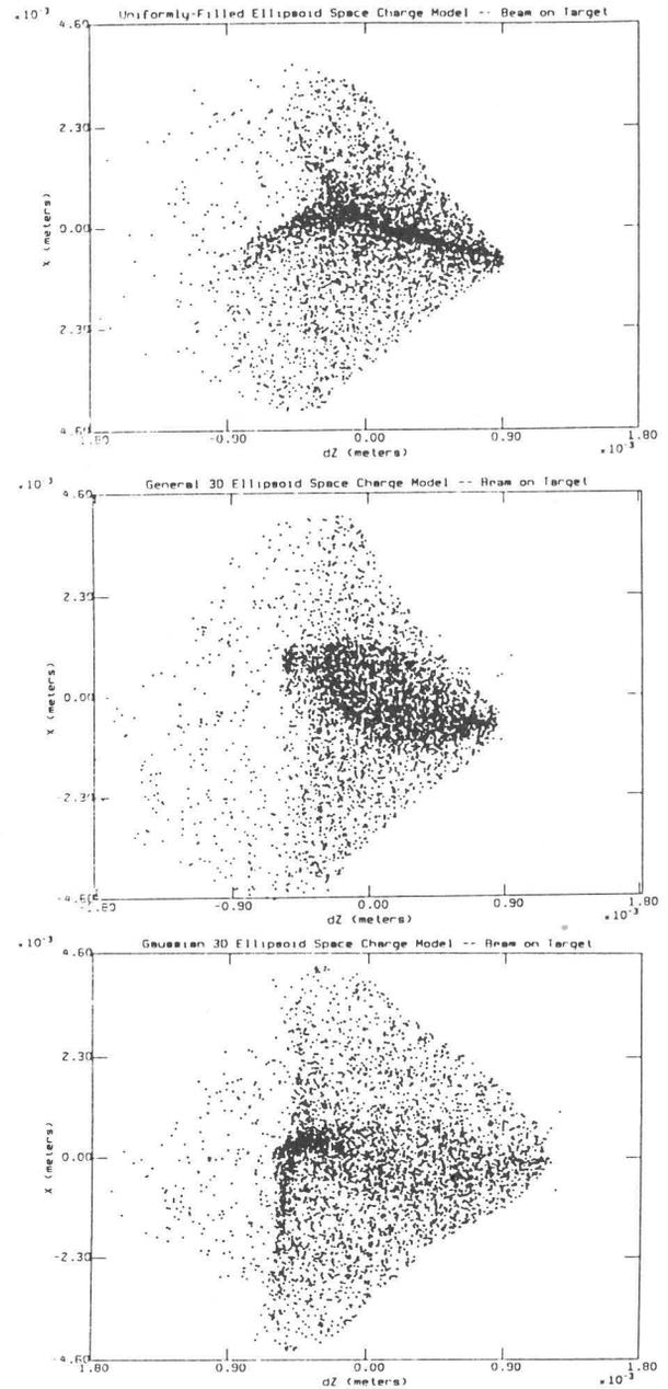
Fig. 5 9 MeV  $e^-$  beam on target using linear (top), G&W (middle) and Gaussian (bottom) space charge models
