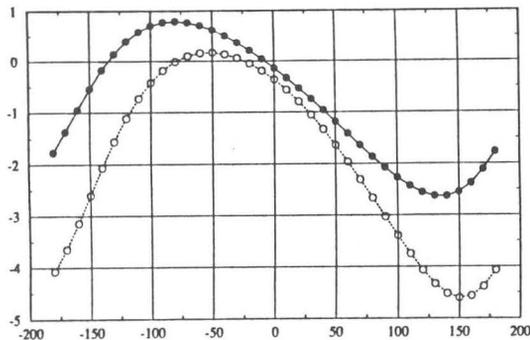
Figure 5 : Beam displacement (mm) for a rf phase variation (deg) of the 3rd module
