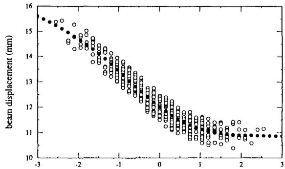
Figure 3 : Transverse profile with 10 mm offset at the exit of the TTF linac ( $N=10^{10}$ )
