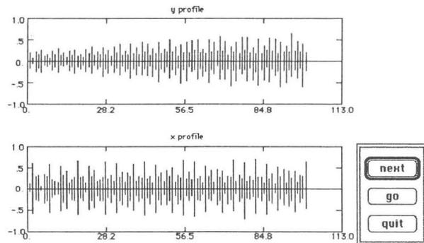
Fig. 3. Vertical and horizontal beam profile displays during the interactive running of PARMILA from the interface.
