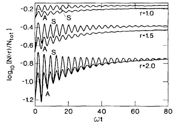
Fig. 4. Fractional number of particles outside  $r=1$  (top),  $r=1.5$  (center), and  $r=2$  (bottom). "S": self-consistent solutions; "A": analytic solutions.
