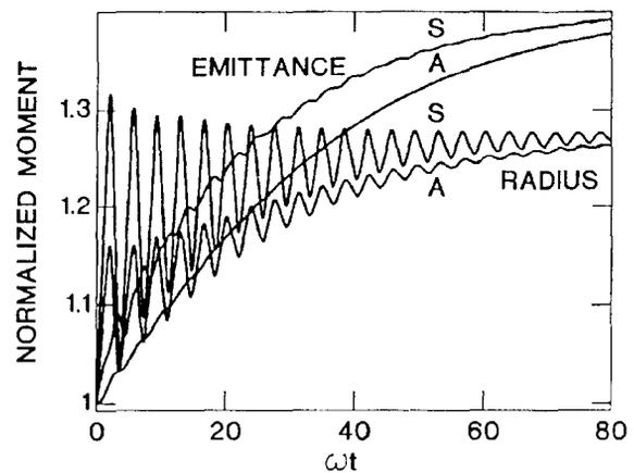
Fig. 3. Rms radius, emittance normalized to  $t=0$ . Self-consistent solutions are denoted "S". Analytic solutions with harmonic-oscillator orbits are denoted "A".
