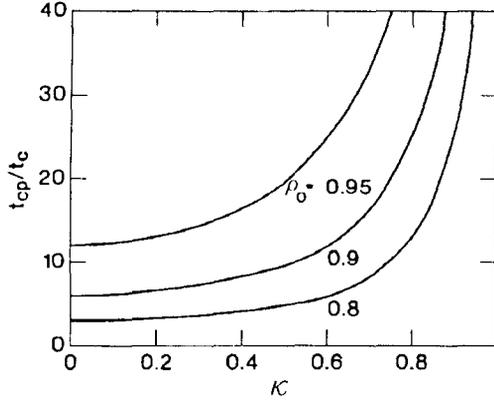
Fig. 1. Plots of  $t_{cp}$  vs.  $\kappa$  for various choices of rms mismatch of a uniform, oscillating core.
