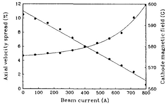
Figure 4. The axial velocity spread as a function of beam current.
