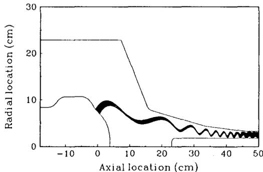
Figure 2. The magnetron injection gun layout.
