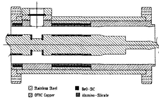
Figure 5. The coaxial second-harmonic circuit.
