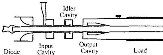
Fig. 1: Schematic diagram of the RKA
