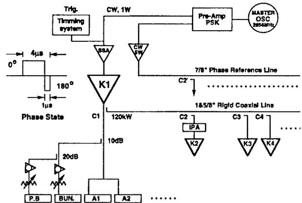
Fig. 1 Klystron power drive system schematic
