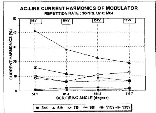
Fig. 4 AC-line current harmonics of the modulator
