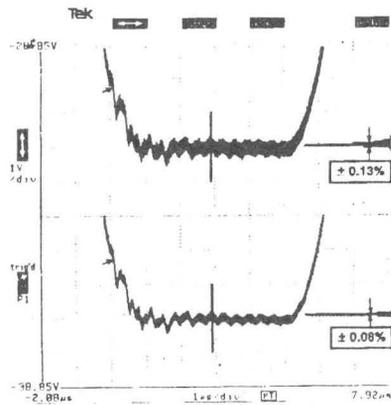
Fig. 5 Accumulated klystron beam voltage fluctuations (flat-top). Upper trace; SCR feedback control only. Lower trace; with De-Q'ing.
