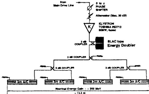
Fig. 2 Microwave power network of a regular linac module
