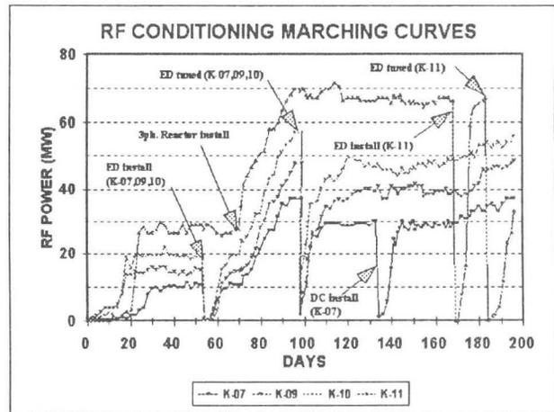
Fig. 7 Typical RF power marching history during the rf conditioning of the accelerating structures and waveguides.
