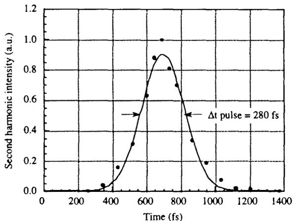
Figure 2: Autocorrelation trace of the IR laser pulse
