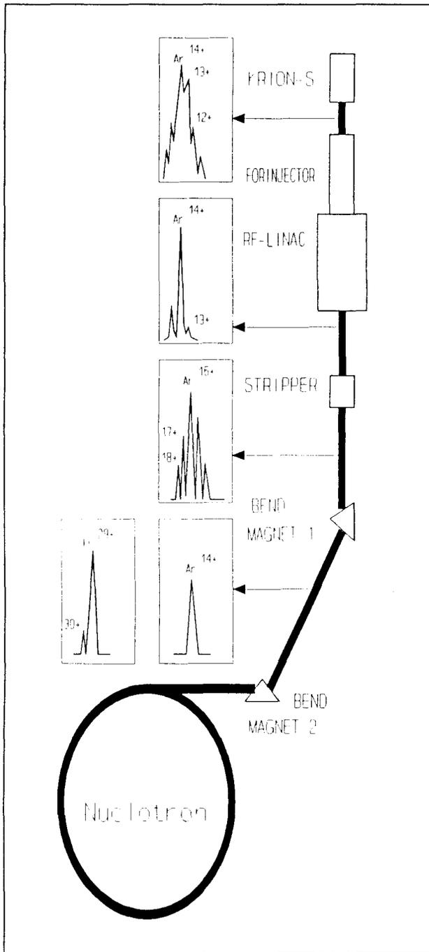
Fig. 2 Accelerating scheme
