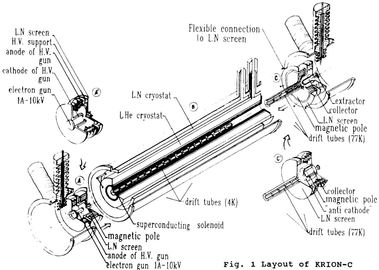
Fig. 1 Layout of KRION-C
