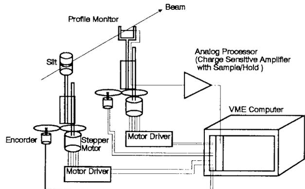
Fig. 1 Emittance monitor used in the preinjector.
