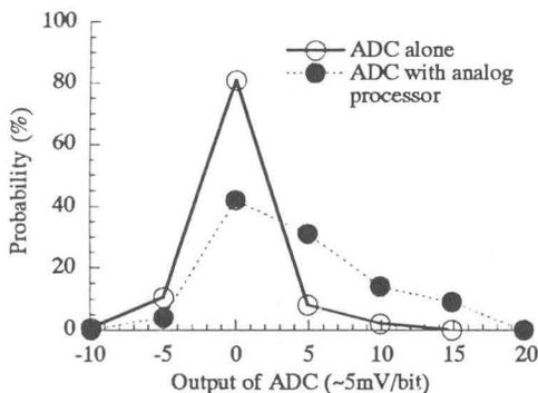
Fig. 5 Probability of ADC output. No signal was inputted. The standard deviation means the noise level. Sensitivity: 1V/pC
