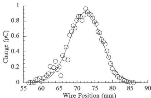
Fig. 4 Beam profile. Beam condition: 1A peak, 0.5ns FWHM and 10MeV
