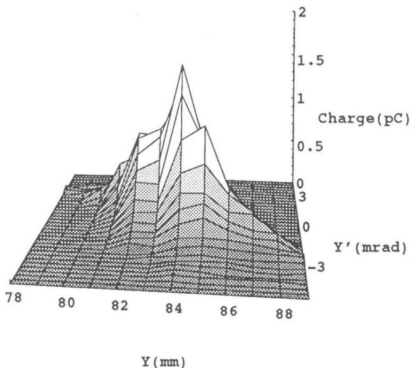
Fig. 6 Density distribution on the phase space. The emittance was obtained as 8.6 $\pi$ mm·mrad. Beam condition: 7.1A peak, 1.5ns FWHM and 12MeV.
