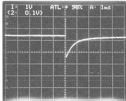
Fig. 2 Output of charge sensitive amplifier in the normal operation. Charge from profile monitor was  $\sim 1.8\text{pC}$ . Sensitivity: 1V/pC
