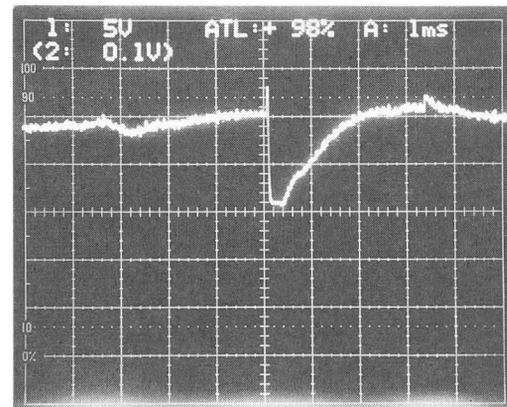
Fig. 3 Output of charge sensitive amplifier when the semirigid cable to the analog processor touched to the modulator frame. Output was saturated. Sensitivity: 1V/pC
