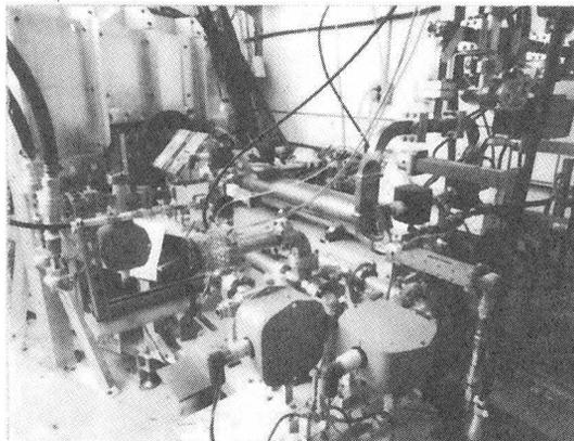
Fig. 2. Experimental setup for high-power tests of the 75 cm traveling-wave section.
