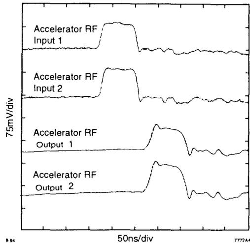
Fig. 9. Input and output RF waveforms for the 1.8 m detuned section at average accelerating gradient of 53 MV/m.
