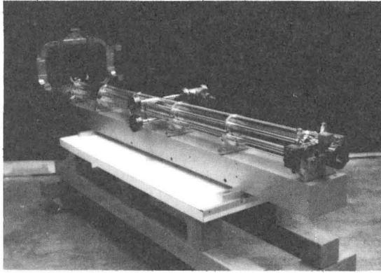
Fig. 3. First 1.8 m detuned accelerator section.
