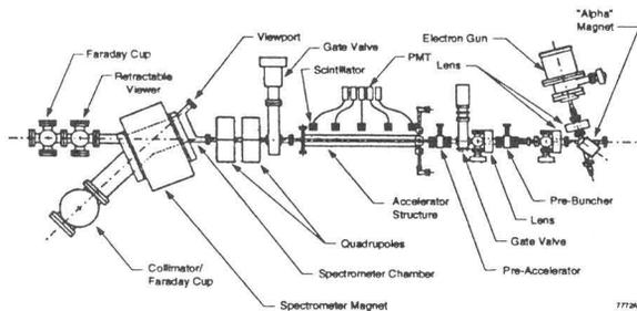
Fig. 1. Layout of the Accelerator Structure Test Area.
