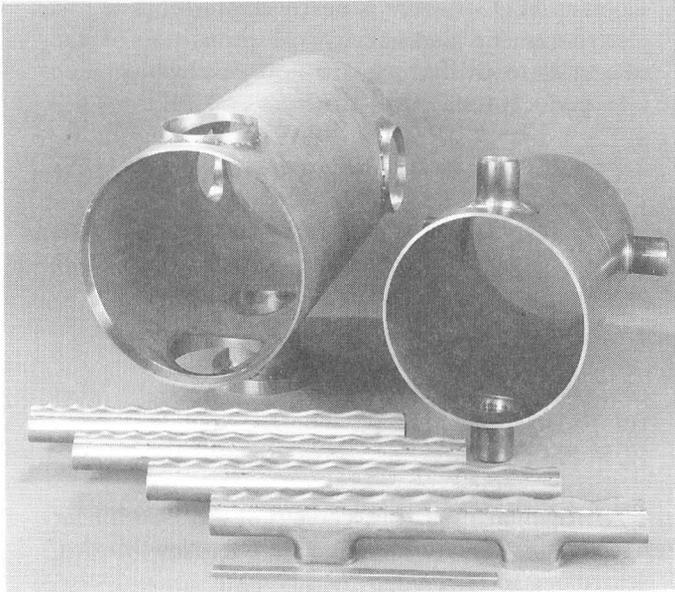
Fig 2 Principal components of the RFQ, including vanes, niobium housing, and stainless-steel outer jacket.
