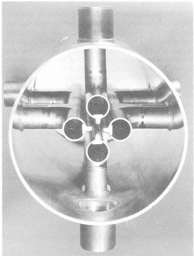
Fig. 1 Major niobium elements of the prototype superconducting RFQ temporarily assembled for tuning prior to final weldment.
