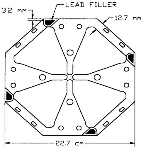
Figure 2: Electroformed 350 MHz RFQ Linac
