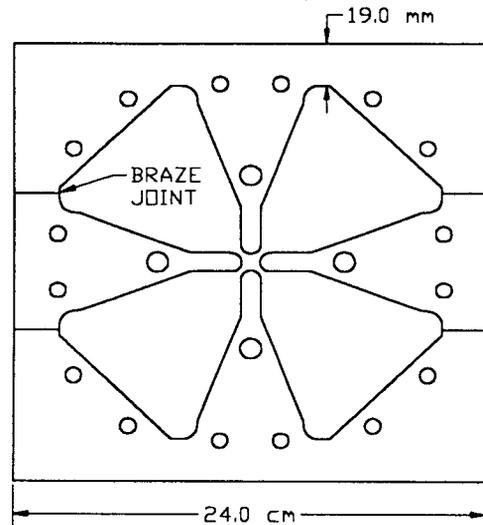
Figure 3: Brazed 350 MHz RFQ Linac
