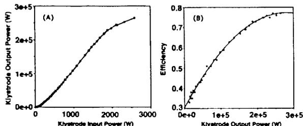
Fig. 4. (A) Output power from the final power amplifier vs. input power. The power gain is greater than 20 dB. (B) Klystrode efficiency vs. output power.
