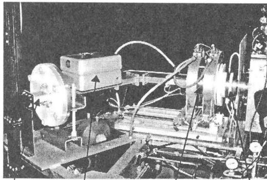
Fig. 2. Photograph of the 50 keV injector installation at Los Alamos.
