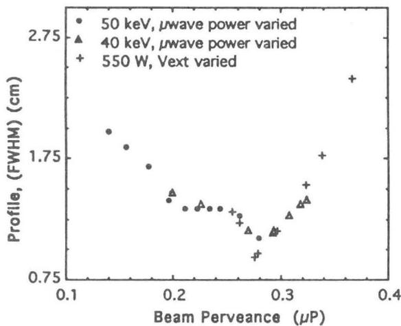
Fig. 3. Plot of the measured beam profiles vs. the beam perveance.
