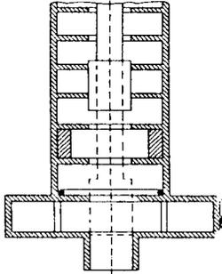
Fig. 2 Schematic drawing of experimental model for measurement of the first DLW cell parameters ( $f_{r1}$ ,  $\frac{k_e}{2}$ )
