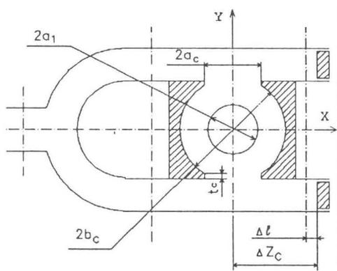
Fig. 1 Schematic geometry of DESY linear collider coupler the DESY linear collider project the coupler version shown
