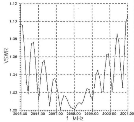
Fig. 4 The impedance characteristic of 6m length accelerating section with ideal tuned cells and matched couplers
