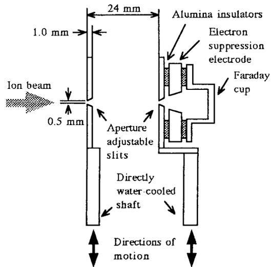
Fig.2 Schematic drawing of the emittance monitor
