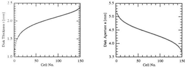
(t): Disk thickness distribution      (a): Disk aperture distribution
