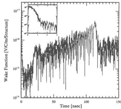
Figure 8: Wake function of the detuned structure.
