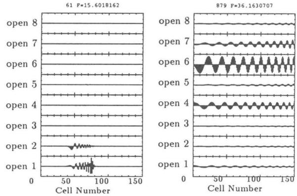
Figure 7: The coefficients of the open mode expansion of the 61'th (15.6GHz, left) and 879'th (36.2GHz, right) modes of the detuned structure.
