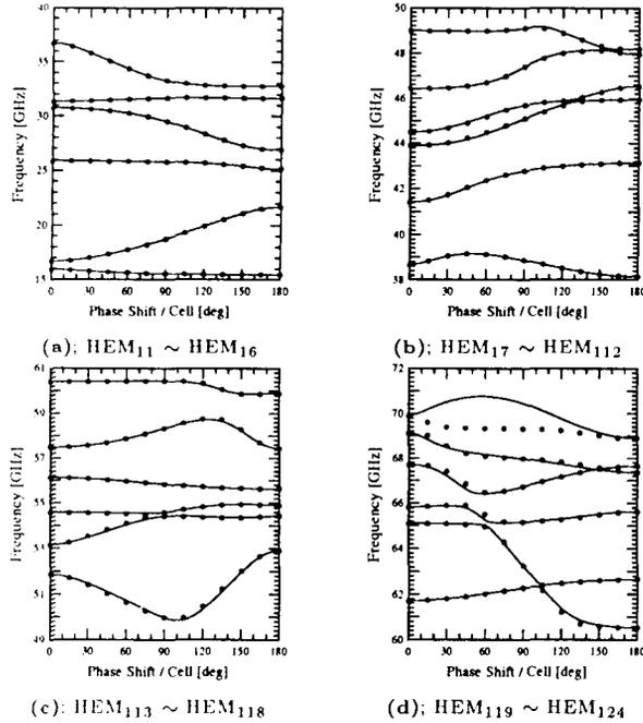
Figure 2: Dispersion relations. Solid lines show the results of the open mode expansion and closed marks show those of the field matching technique.
