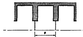
Figure 1: Cell geometry of infinitely periodic structure.
