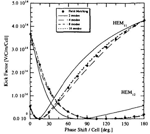
Figure 3: Kick factors of the two lowest modes. Lines show the results of open mode expansions with various numbers of modes. The closed circles show those of the field matching.
