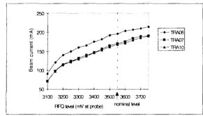
Fig. 3 Linac 2 currents as function of RFQ level
