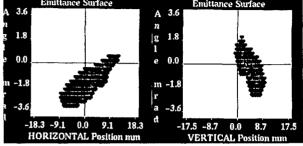
Fig. 4 Measured Linac 2 Horizontal and Vertical Emittances
