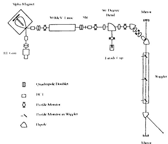
Fig.1 Schematic layout diagram of BFEL
