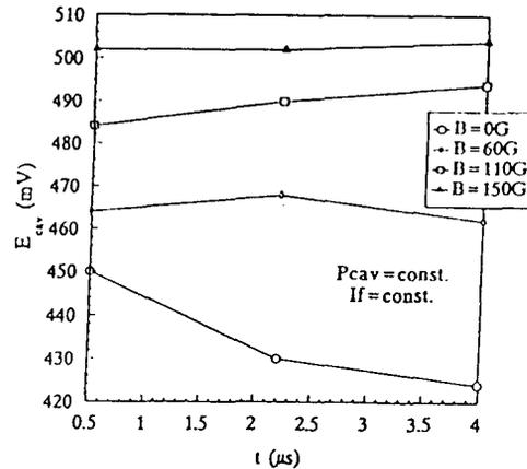
Fig. 2 Cavity field vs. time at different deflecting field.
