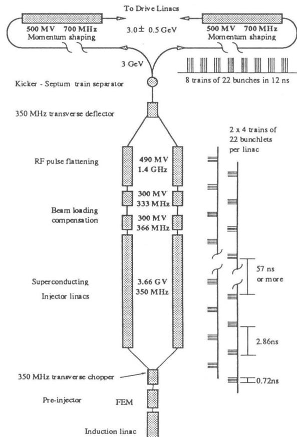
Fig. 5 Possible layout for FEM drive beam generation
