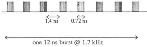
Fig. 2 Drive beam time structure
