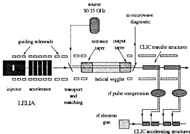
Fig. 6 Layout of the CLIC Test Section Experiment
