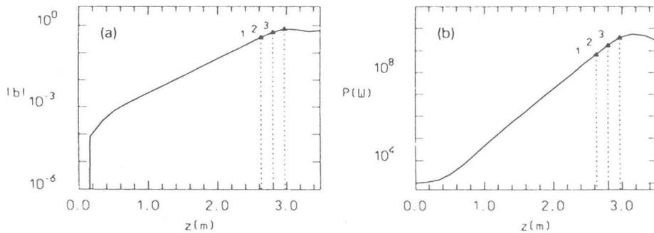
Fig.3 Simulation of the FEL process. We show: (a) the bunching parameter  $|b_1|$ , proportional to the 30 GHz Fourier component of the beam current and (b) the output microwave power in Watts, in a logarithmic scale, as a function of the length of the wiggler,  $Z$  (m). For an explanation of the marked points refer to Fig. 4.
