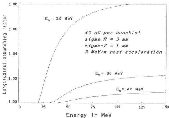
Fig. 6 Bunch lengthening due to space charge during post-acceleration.
