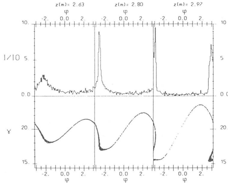
Fig. 4 Phase histogram, showing the electron current in a wavelength (top) and electron distribution in the longitudinal phase space (bottom), at three different locations.  $I_0$  is the average input electron current. Note the strong peak current (bunching) that can be obtained if one stops the interaction at the proper point ( $Z = 2.84$  m). The three pictures corresponds at the points marked in Fig. 3.
