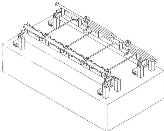
Fig. 1 A 1.4 m long module of CLIC. To the right are shown two transfer structures feeding the four accelerating structures to the left. The 30 GHz power is generated by the drive beam traversing the transfer structures.
