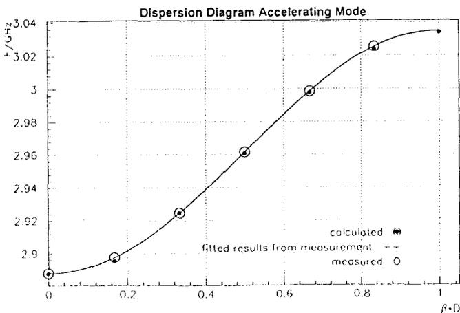
figure 4: dispersion diagram of the accelerating mode passband including the frequencies calculated by mafia.
