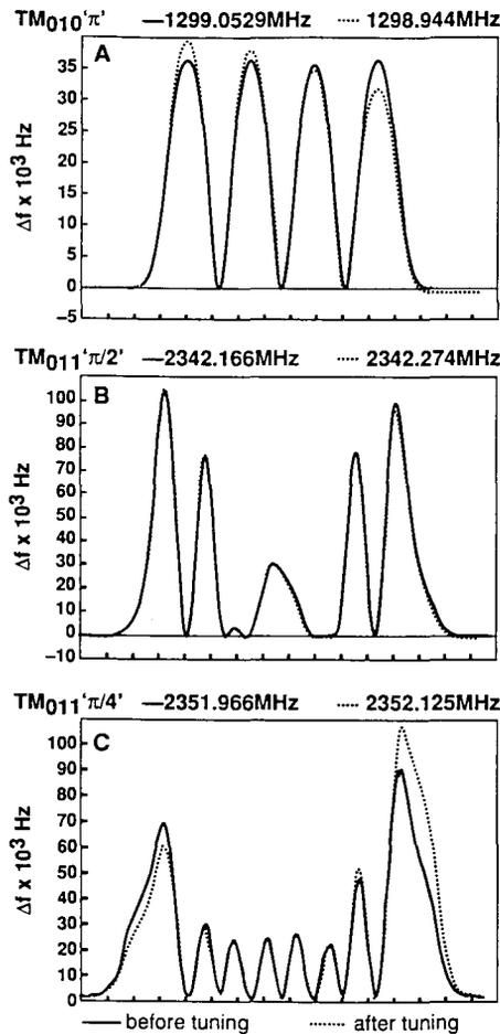
Fig. 4. Profiles of selected longitudinal modes before and after end cell tuning.
