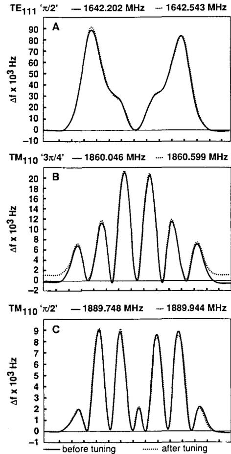
Fig. 5. Profiles of selected dipole modes before and after end cell tuning.
