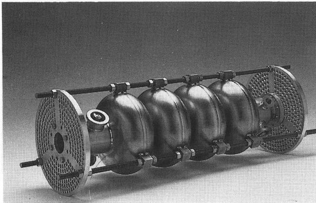
Fig. 1. Four cell CERN/DESY structure with longitudinal rods and end plates.
