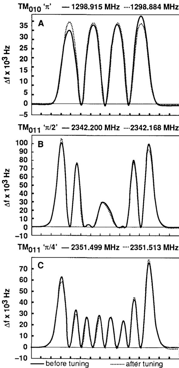
Fig. 2. Field profiles of some longitudinal modes before and after tuning of the accelerator mode(2a).
