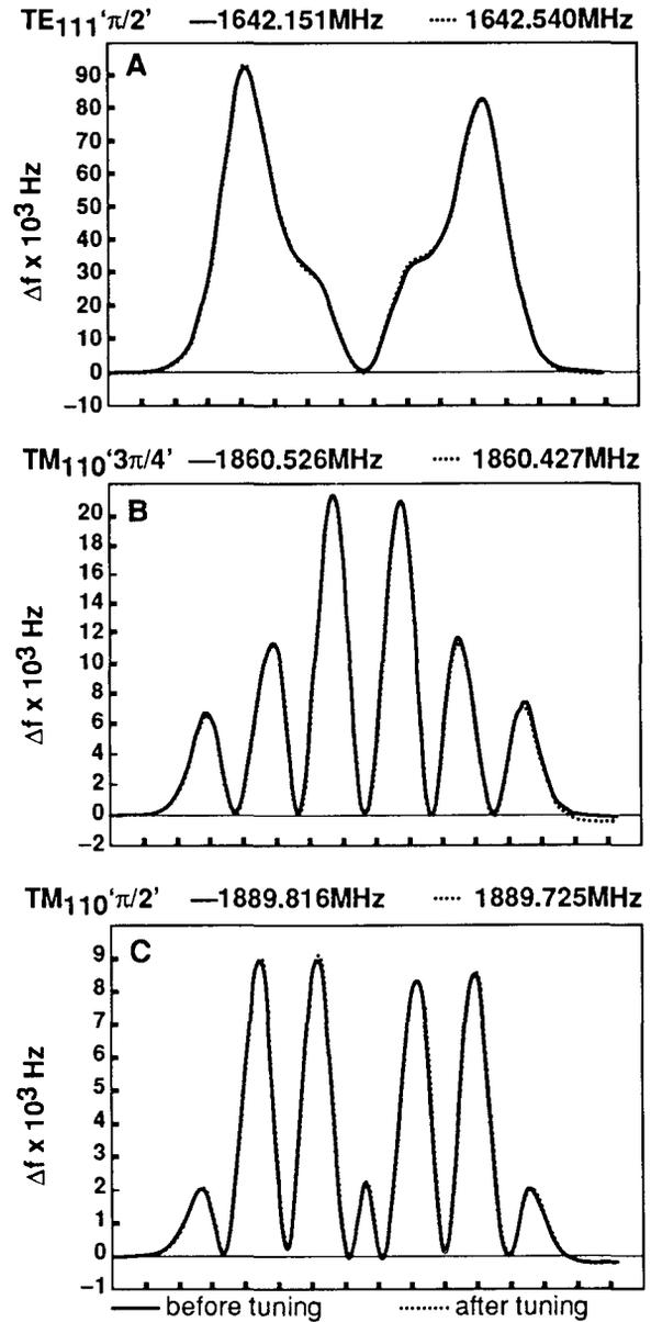
Fig. 3. Field profiles of some dipole modes before and after tuning of the accelerator mode.
