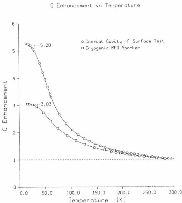
Figure 2 - Cryogenic Cavity Q Enhancement.
