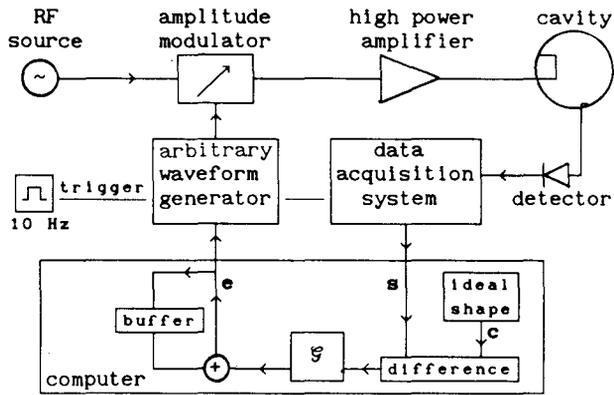
Fig.4. Function feedback loop.
