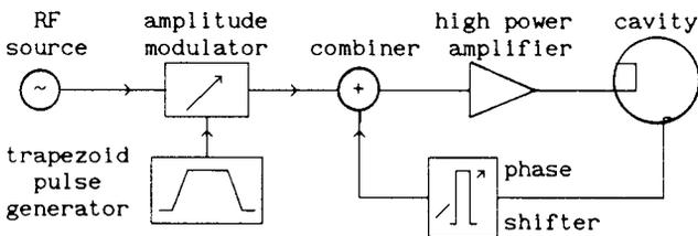
Fig.1. Analog RF feedback loop.
