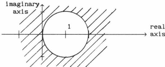
Fig.3. Stability area for  $\mathcal{G}\mathcal{F}$  operator.
