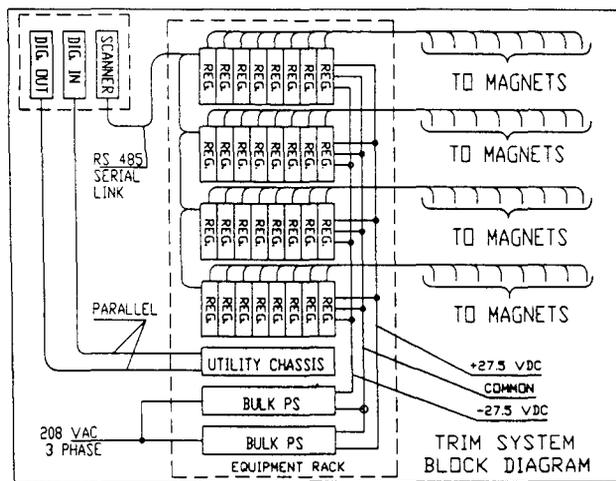
Figure 1. Trim System Block Diagram.
