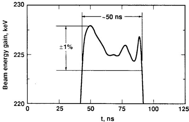
Figure 8. ETA-II "Two-cell" Acceleration Gap Voltage Pulse.  $I_{beam} = 2.13$  kA.
