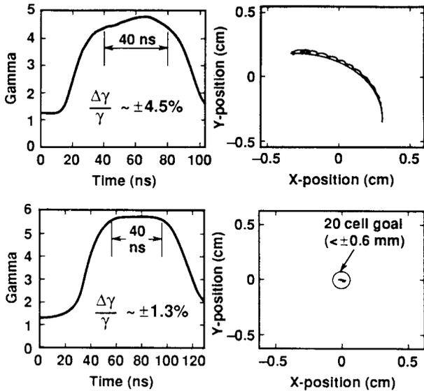
Figure 6. BREAKUP Simulations. Corkscrew motion is plotted for 40 ns as shown in each accompanying plot. ETA-II simulations for previous bus (top). Simulations of expected results (bottom),  $dE/E = \pm 1.3\%$ .
