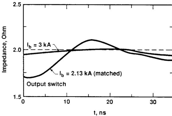
Figure 7. Optimum impedance tapers for specified beam currents.
