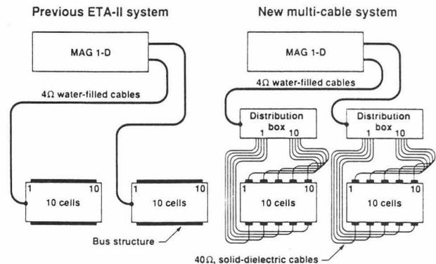
Figure 2. ETA-II Modifications. Previous ETA-II bus structure (left). Modified ETA-II "two cell" bus structure (right).
