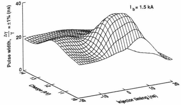
Figure 5. ETA-II 20 Cell Experiment Pulse Width Optimization Surface. Pulse width values are for  $dE/E = \pm 1\%$ ,  $I_{beam} = 1.5 \text{ kA}$ .
