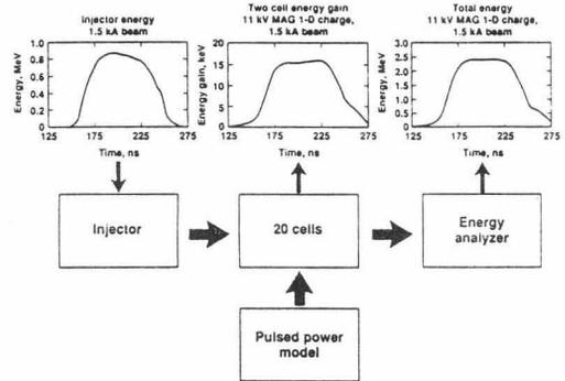
Figure 4. Compensation of the ETA-II 20 cell experiment.
