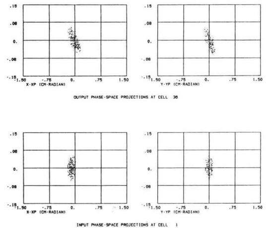
Figure 5. Input and output phase space plots of the HESQ for a misaligned injected beam
