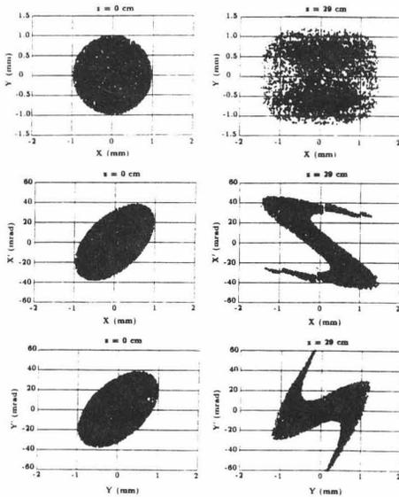
Figure 3: Phase-space plots of the particle distribution from the PARMILA code at the beginning and end of the six-quad ESQ system.
