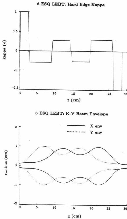
Figure 1: Hard-edge variation of the focusing function  $\kappa(z)$  at top and beam envelopes  $X(z), Y(z)$  at bottom.
