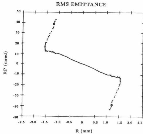
Figure 5: Phase space distribution of the laminar beam from the SNOW code at  $z = 22.2$  cm.
