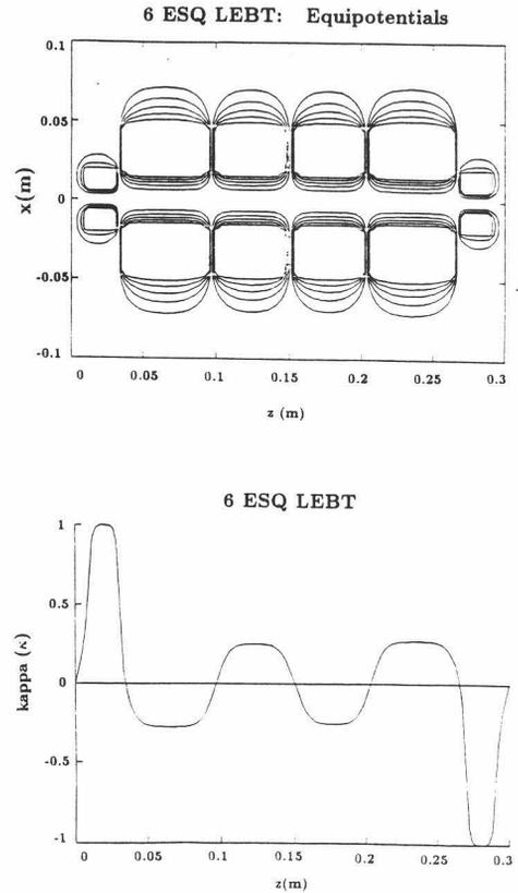
Figure 2: Geometry with potential distribution of ESQ system (top) and variation of  $\kappa(z)$  along  $z$ -axis (bottom).
