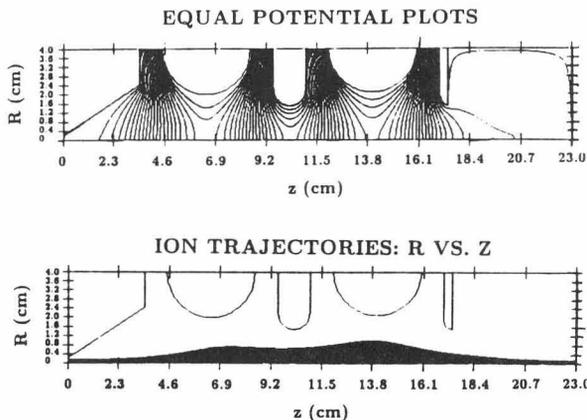
Figure 4: Electrode configuration of the einzel lens system with potential distribution (top) and beam profile (bottom) from the SNOW code.
