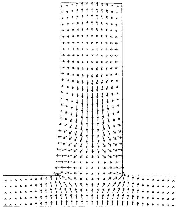
Fig. 5. Electric field pattern for axially asymmetric ( $p=1$ ) pillbox mode when  $w/b = 2.4$ . Note that this mode is *not* evanescent into the radial line, but is evanescent into the beampipe. Resonant frequency of this mode is 5.18 GHz.
