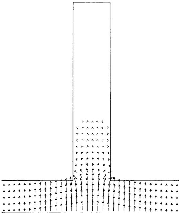
Fig. 4. Electric field pattern for lowest frequency axially asymmetric mode when  $w/b = 1.4$ . Note that the mode is evanescent into the beampipe and into the radial line. Resonant frequency of this mode is 5.42 GHz.
