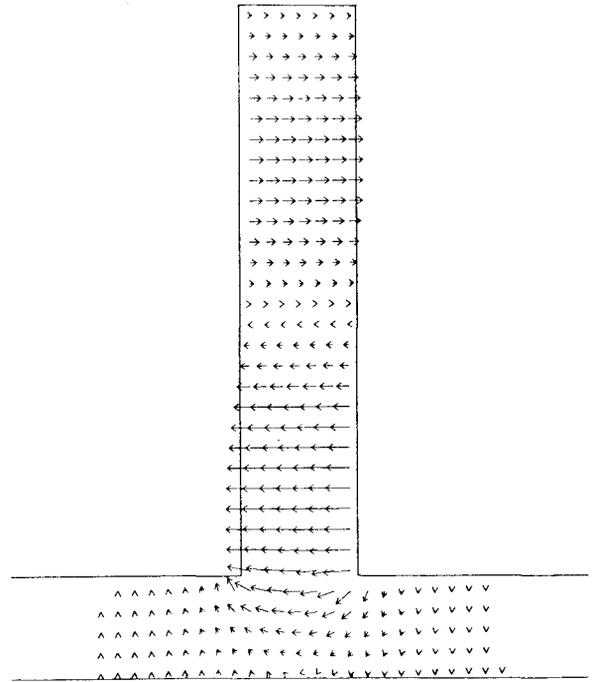
Fig. 3. Electric field pattern for 3.3 GHz axially symmetric mode when  $w/b = 1.4$ .
