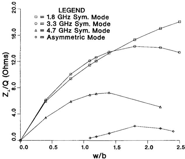
Fig. 2. Variation in  $Z_{\perp}/Q$  with  $w$  for first (lowest frequency) three axially symmetric dipole modes and the first asymmetric dipole mode. Result is for  $r = r_Q = b$ , and  $\phi = 0$ .
