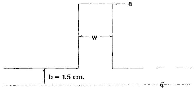
Fig. 1. Rotationally symmetric "Briggs pillbox" used in all calculations presented in this paper. Pillbox is terminated with a perfect conductor. Beampipe was long enough so that the beampipe terminations did not affect calculated results (considered only modes with resonant frequencies less than the beampipe cutoff). Pillbox radius  $a = 6.7b = 10.05$  cm.
