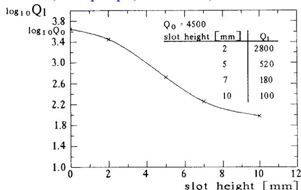
Fig. 9  $Q_1$  versus slot height, ( $Q_1 = Q_0 / (1 + k)$ )
