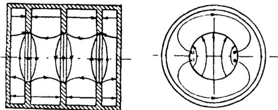
Fig. 1  $TM_{110}$   $\pi$ -mode, E- and H- field plot
