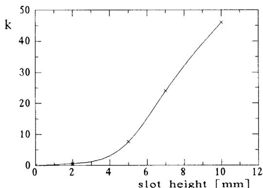
Fig. 8. Coupling factor versus slot height
