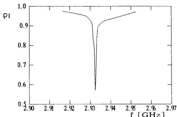
Fig. 6 Reflection coefficient versus frequency for a 5mm slot
