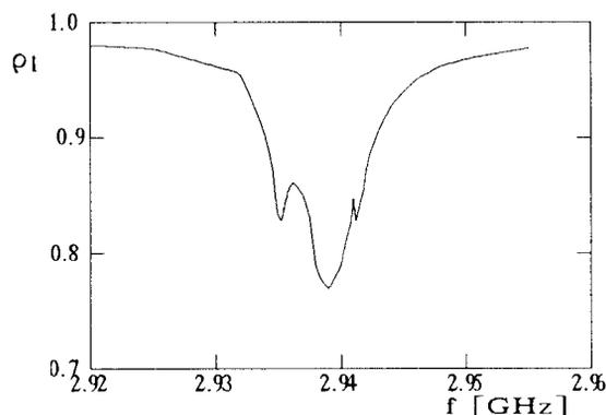
Fig. 7 Reflection coefficient versus frequency for a 2mm slot
