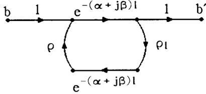
Fig. 4 Signal flow plot of the experimental setup
