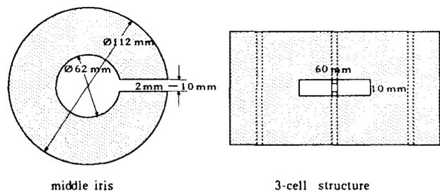
Fig.3 Coupling slot geometry
