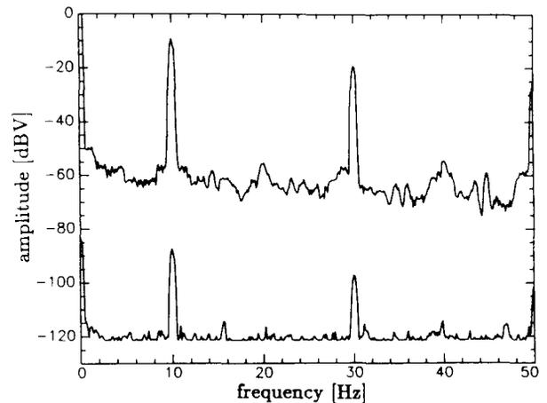
Fig. 3 Spectrum of Amplitude Error Signal in Open and Closed Loop Cases
