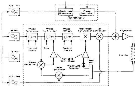
Fig. 1 RF System Schematic
