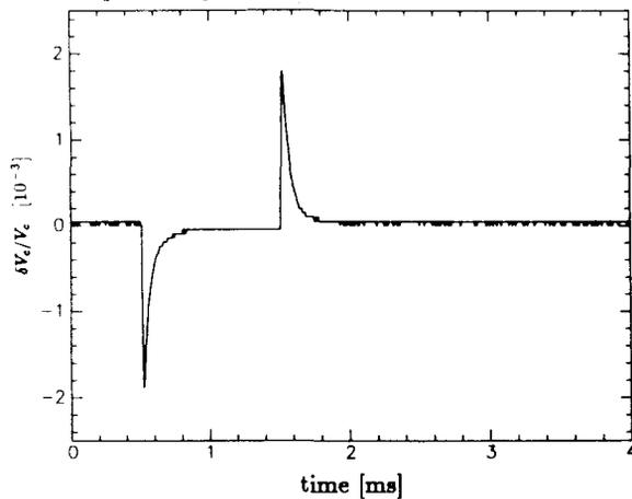
Fig. 5 Transient Amplitude Error Signal from Beam
