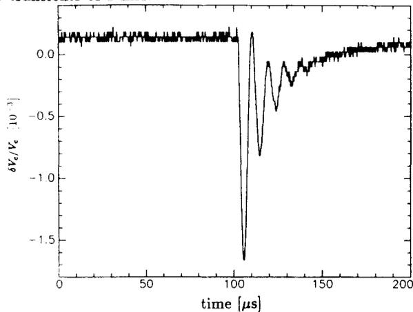
Fig. 4 Transient Amplitude Error Signal from Beam Box
