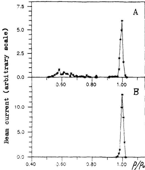
Fig.4. Spectrum of the output beam at the buncher off (A) and on (B)
