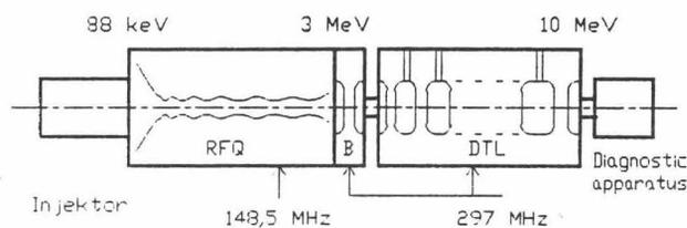
Fig.1. Block diagram of the Linac Istra-10.
