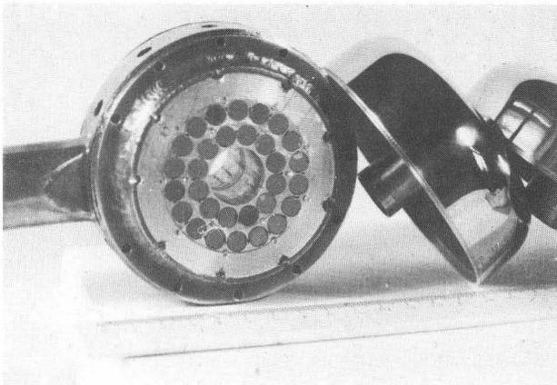
Fig.3 Open into vacuum the drift tube with PMQ (before assembling)
