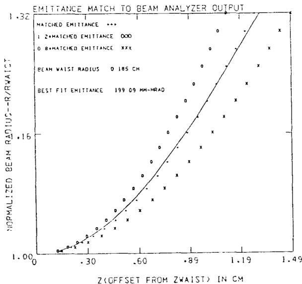
Fig.6. Emittance determination by a match of theoretical relation (Eq.5) to a polynomial representation of beam radius data (continuous curve) for the gridded gun.
