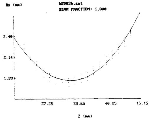
Fig. 2. Beam profiles for the gridded gun. Points with error bars represent data, the solid line is the fit polynomial.
