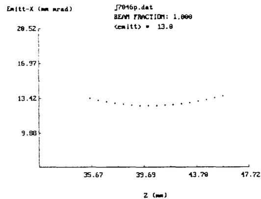
Fig. 3. Emittance of the diode gun as a function of  $z$ .
