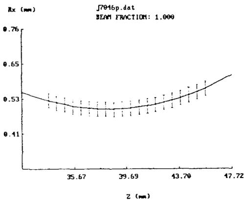
Fig. 1. Beam profiles for the diode gun. Points with error bars represent data, the solid line is the fit polynomial.
