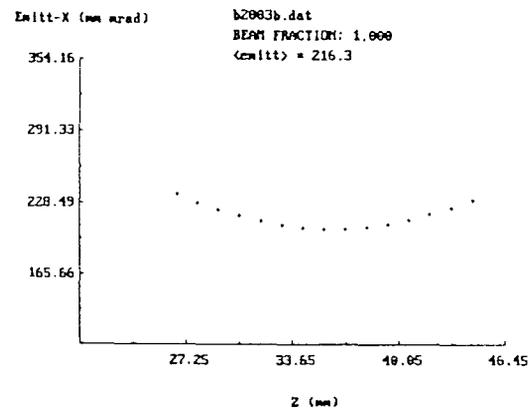
Fig. 4. Emittance of the gridded gun as a function of  $z$ .
