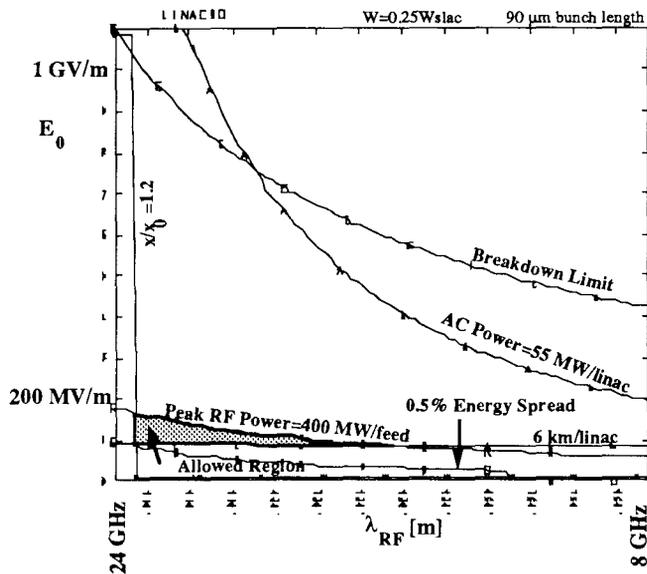
Fig. 2 Accelerator Parameter Space Using Largest Allowed ( $\sigma_y$ - $\sigma_z$ ) From Fig. 1.
