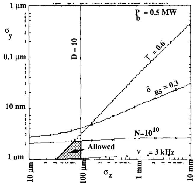
Fig.1 Interaction Point Parameter Space for a 1 TeV (CM) Collider with L=2x10<sup>37</sup> m<sup>-2</sup>·s<sup>-1</sup>.
