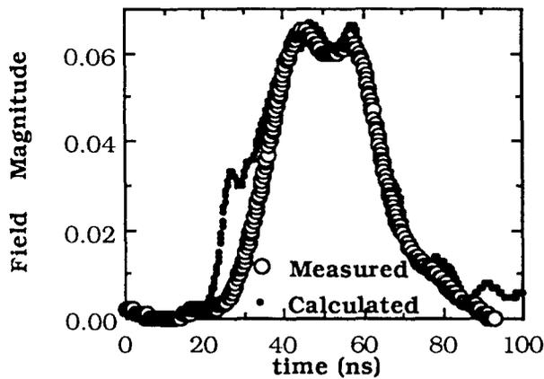
Fig. 1. Comparison of predicted to measure output pulse for the HGA in the RK experiments.
