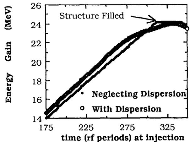
Fig. 3. Energy gain as a function of injection time.
