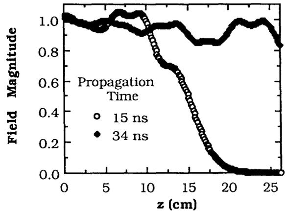
Fig. 2. Accelerating field along axis of a HGA.
