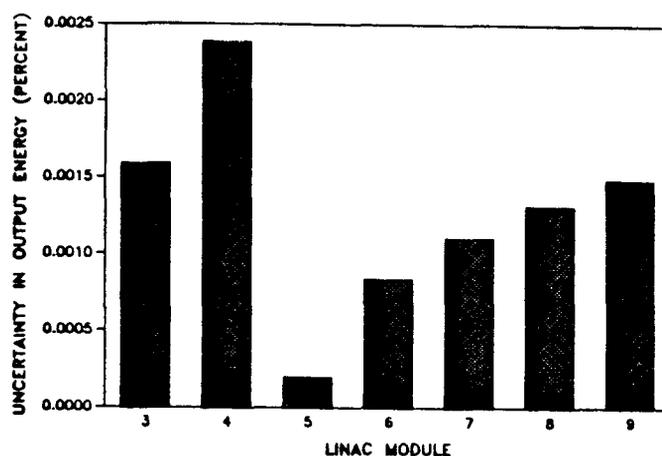
Figure 6. Uncertainty in output energy for the high-energy delta-t procedure in the Fermilab linac. One picosecond random errors in delta-t measurements are assumed.
