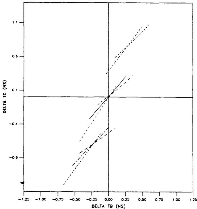
Figure 2. Theoretical delta-t curves for module 5. For the upper curves, input beta=0.41331; for the center curves, input beta=0.41414; and for the lower curves, input beta=0.41497. Electric fields are varied  $\pm 5\%$  about nominal within each cluster.
