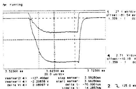
Fig. 2. Waveforms observed on the emittance scanner face and analyzed beam Faraday cup. The upper trace is the scanner face current while the lower trace is the analyzed current pulse shape.
