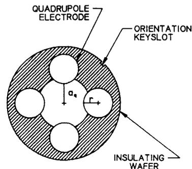
Fig. 3. End view of a HESQ cell. The radius of the electrodes,  $r$ , is 1.0 cm. The radius of the available aperture,  $a_q$ , is 1.3 cm.
