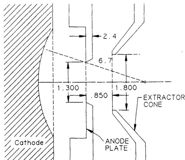
Fig. 1. Extraction geometry (not to scale) for 28 mA source. All dimensions are given in millimeters.
