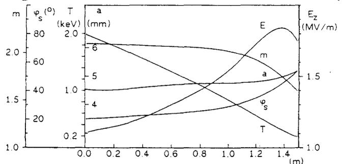
Fig. 3 Electrode design of the decelerating RFQ
