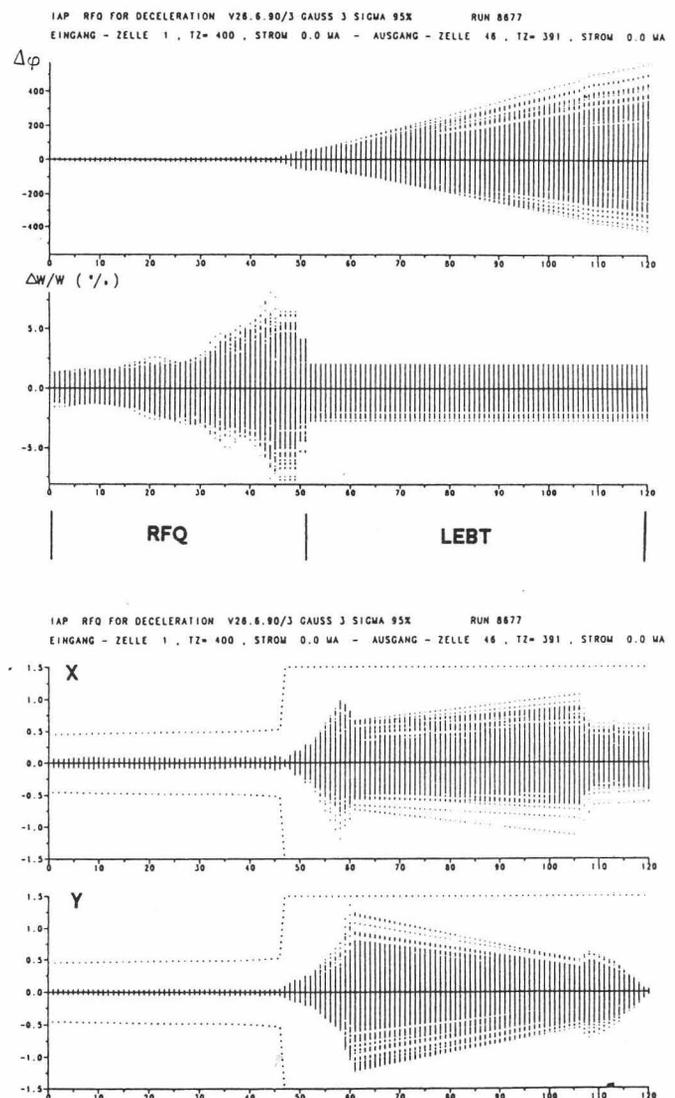
Fig. 5 Example of Parmteq simulation for RFQ and LEBT
