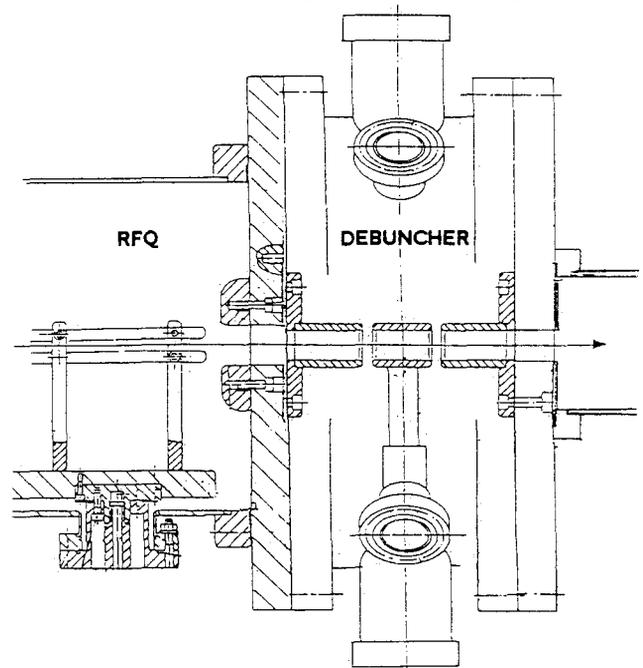
Fig. 2 Scheme of the low energy end of the RFQ
