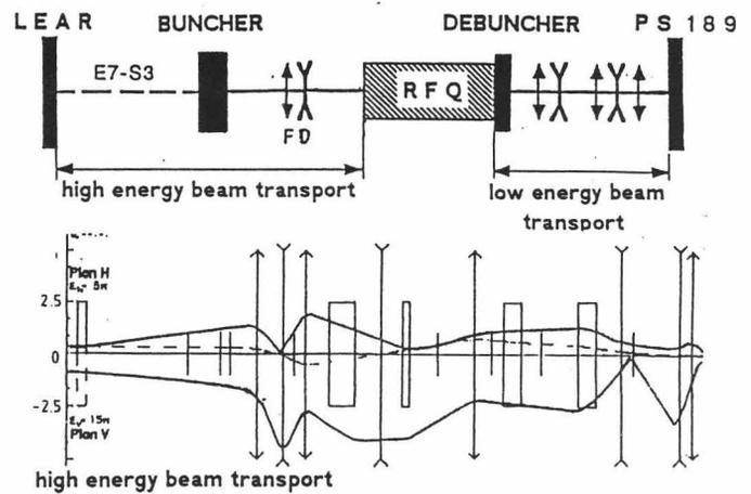
Fig. 4 HEBT for the PS189 experiment
