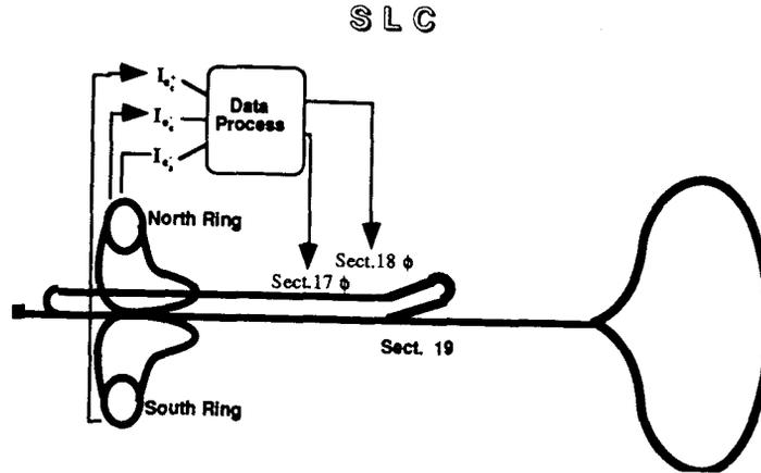
Fig. 2 The feedforward loop to stabilize the scavenger beam energy.
