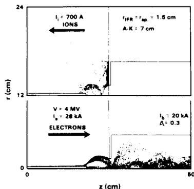
Fig. 8: Foilless apertured diode focused with the positive ions emitted from the anode plasma sheathe
