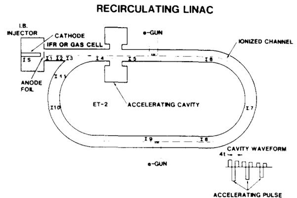
Fig. 1: Schematic diagram of the RLA. Closed racetrack channel configuration.
