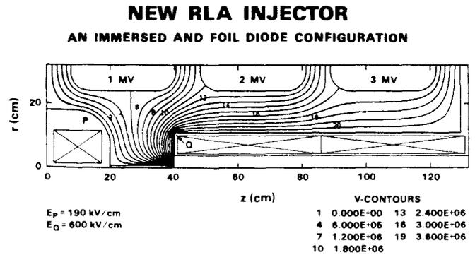
Fig. 5: Schematic diagram showing how the same hardware can accommodate two types of diodes: magnetically immersed and foil diodes.
