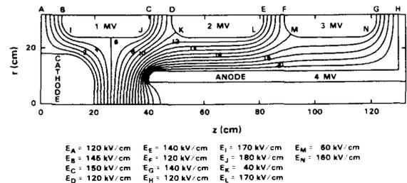
Fig. 2: The new 4-MV RLA injector cavity design and equipotential plots. The magnetically non-immersed foilless diode geometry is also shown.
