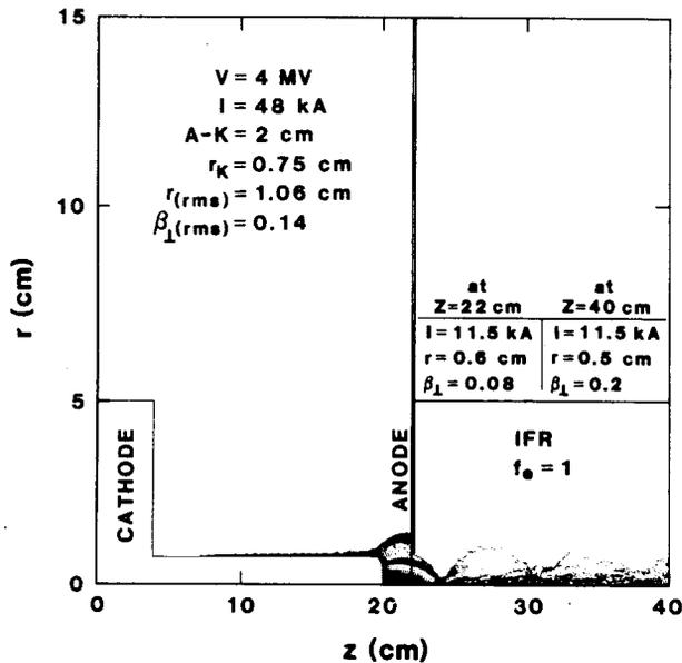
Fig. 7: 4-MV foil diode electron map.
