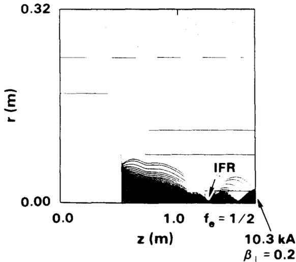
Fig. 4: Electron trajectories for a 4-MV, 10-kA beam.
