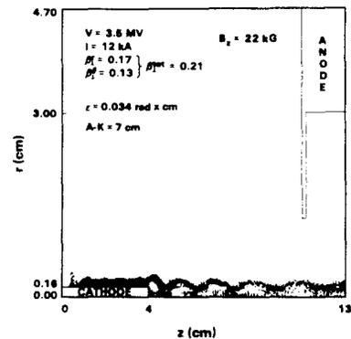
Fig. 6: The magnetically immersed foilless diode produces a low emittance beam.
